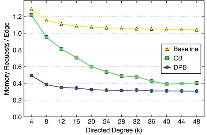
Figure 8. Communication efficiency for uniform random graphs of 128M vertices and varied degree. DPB is best for sparse graphs.
