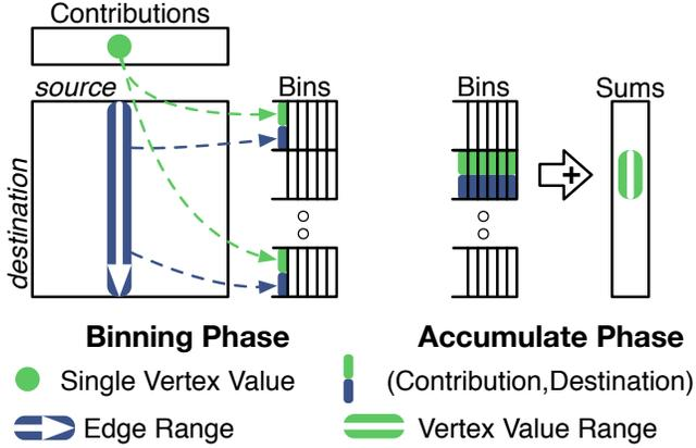
Figure 2. *Propagation blocking*. In the binning phase, vertices pair their contributions with their destination indices and insert them into the appropriate bins. In the accumulate phase, the contributions are reduced into the correct sums.
